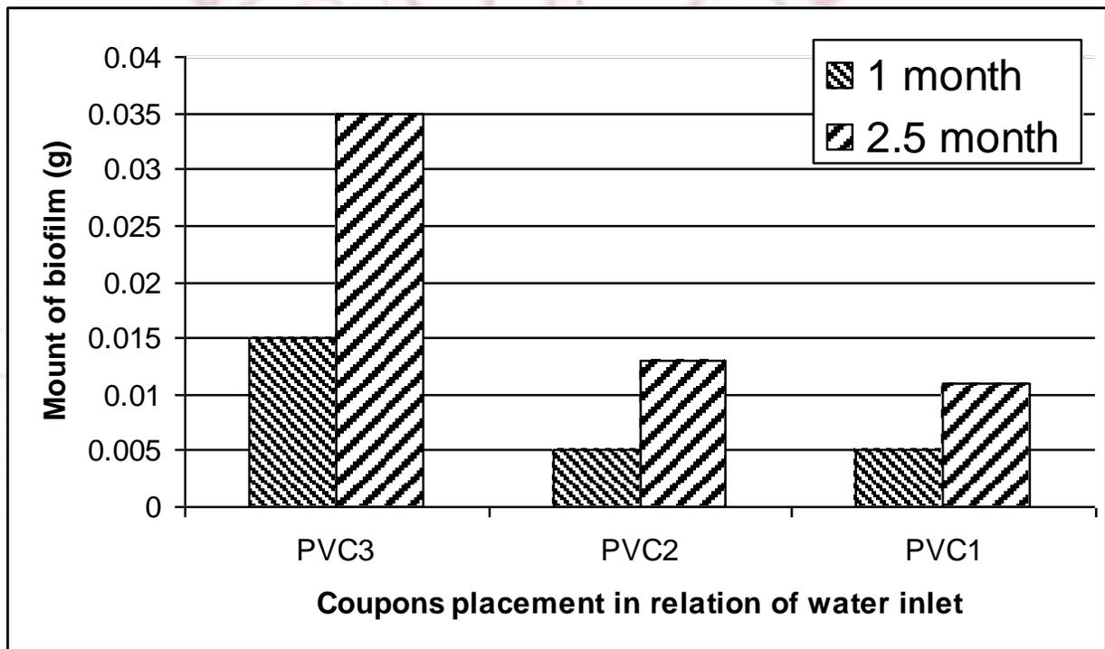
Figure 17. Biofilm growth on PVC coupons with scale.
