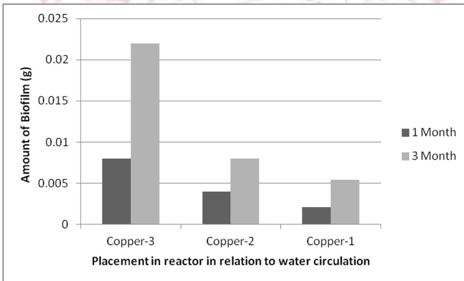
Figure 20. Biofilm growth on copper coupons with soft scale.
