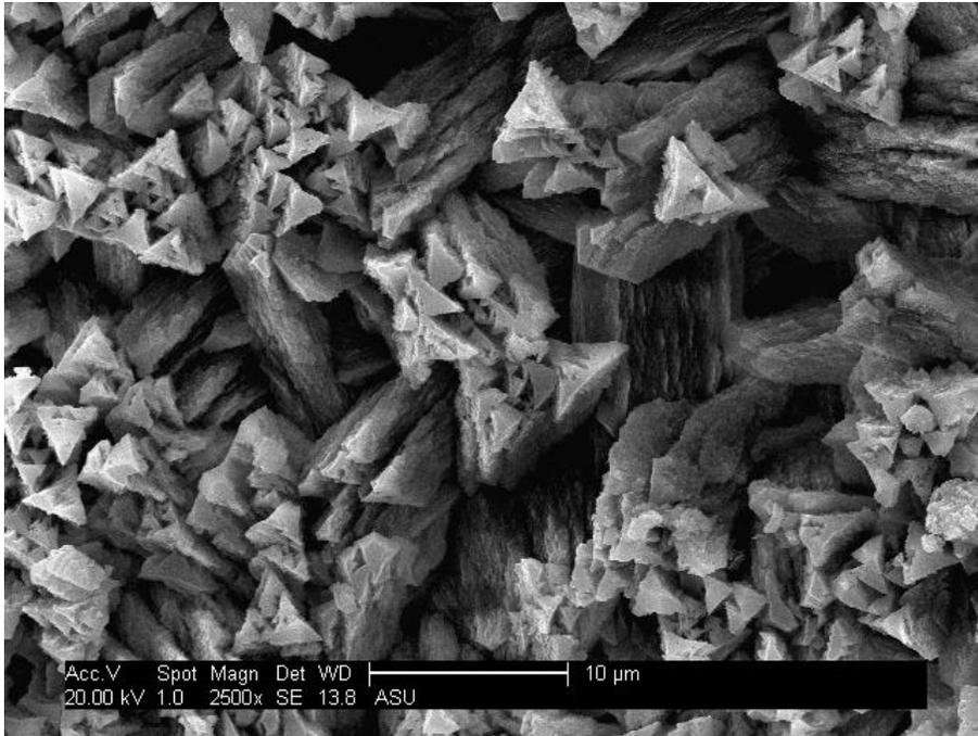
Figure 4. Electron Micrograph of “hard” scale. The calcite crystals are aligned as scale formed directly on the surface.
