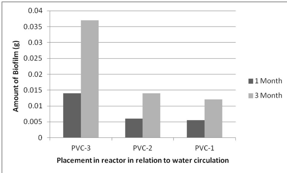
Figure 19. Biofilm growth on PVC coupons with soft scale
