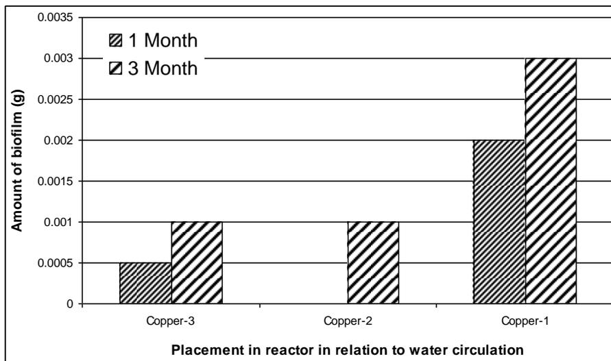
Figure 13. Biofilm formation on copper coupons during testing without iron.
