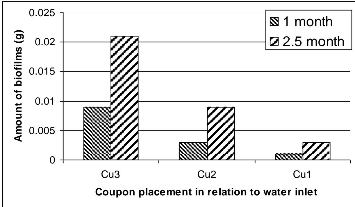
Figure 18. Biofilm growth on copper coupons with scale.
