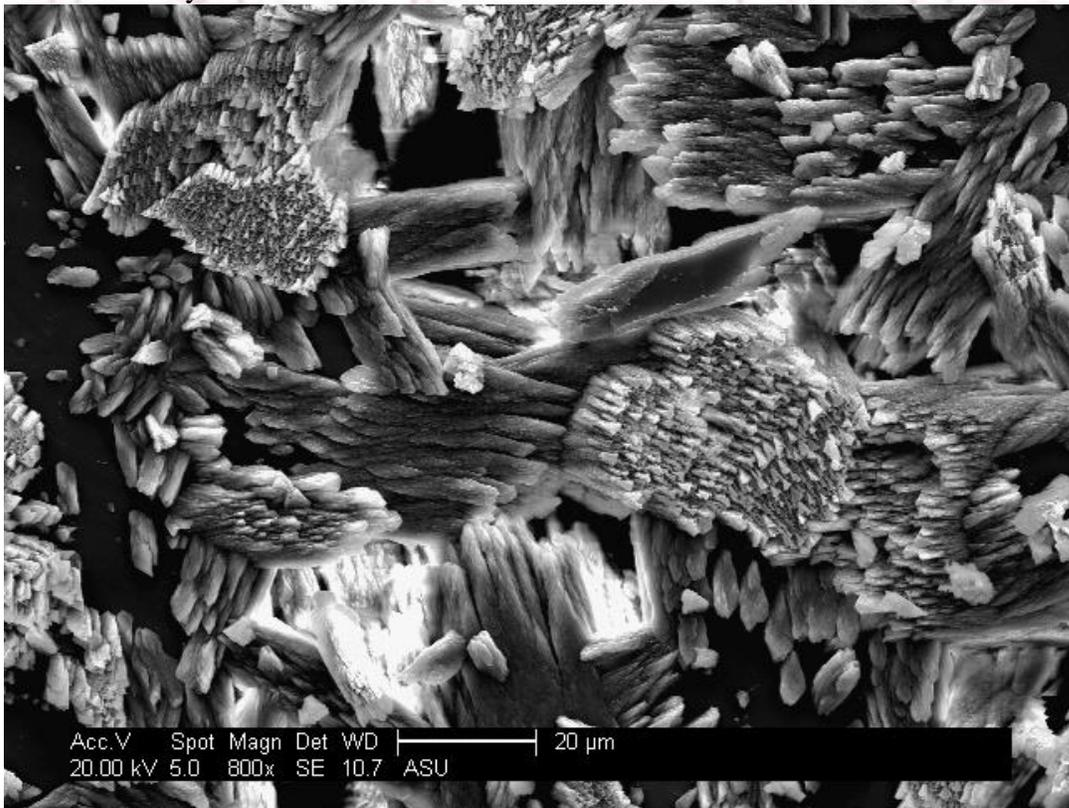
Figure 5. Electron Micrograph of “soft” scale. The calcite crystals are not aligned as deposition occurred on the surface during scale formation.
