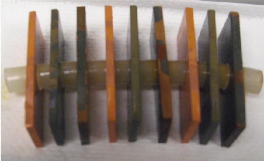
Figure 3. Sequence of Clean Coupons Placed in Recirculating Reactor
