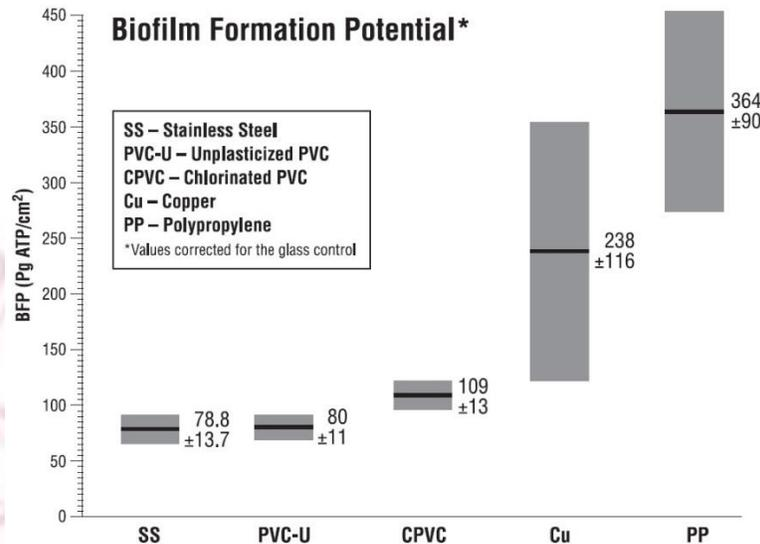
Figure 1. Biofilm formation Potential in different pipe material [40]
