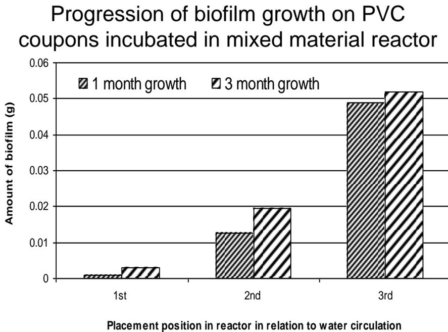
Figure 6. Biofilm Growth on PVC coupons.
