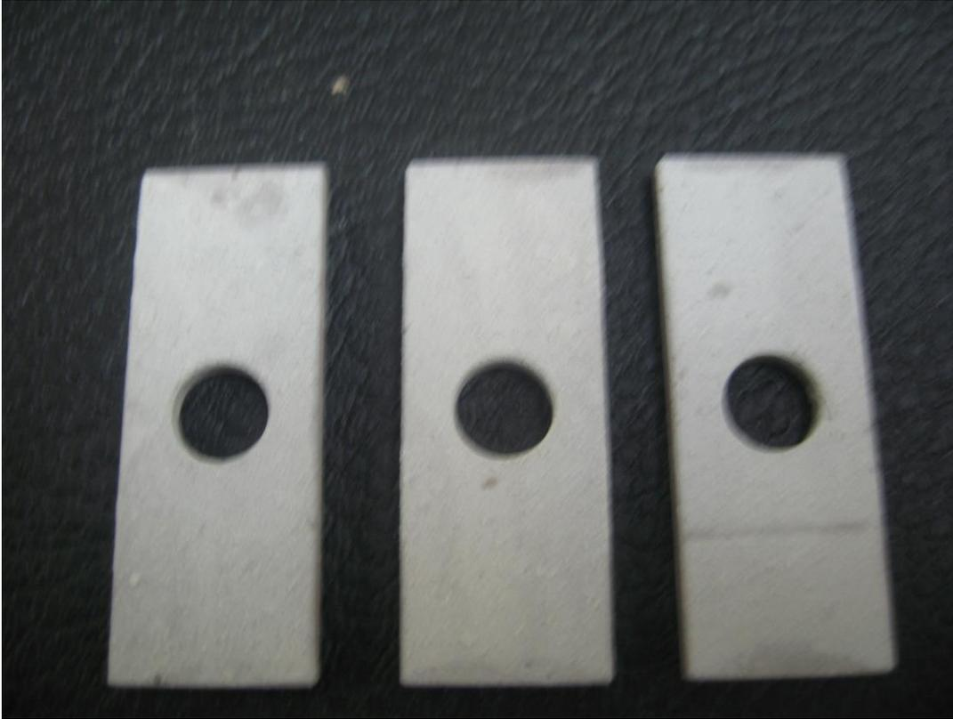
Figure 15. Copper coupons with scale.
