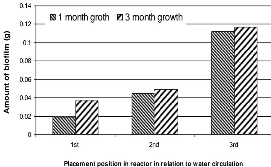
Figure 7. Biofilm growth on copper coupons.
