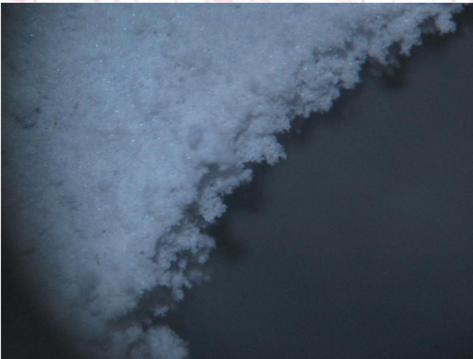
Figure 16. Optical microscope picture of calcite crystals along the center of a coupon.
