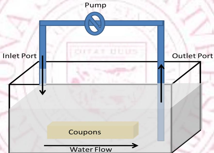
Figure 2. Schematic of biofilm reactor
