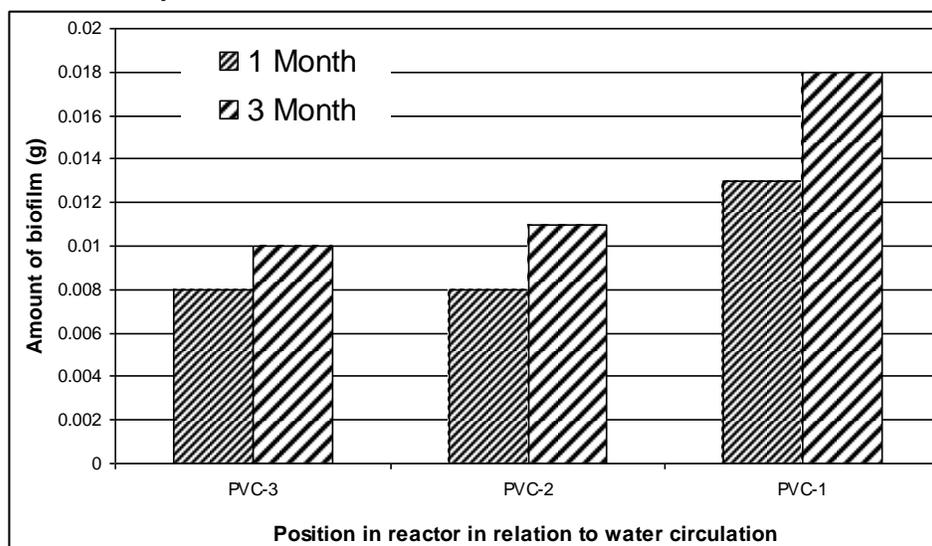
Figure 14. Biofilm formation on PVC coupons during testing without iron.
